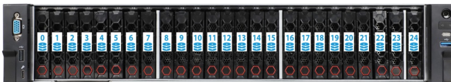
Figure 13 Drive numbering for front 25SFF drive configurations
