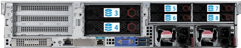
Figure 16 Drive numbering for rear 2LFF+4SFF drive configurations
