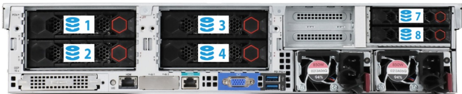
Figure 17 Drive numbering for rear 4LFF+2SFF drive configurations
