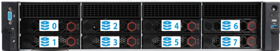
Figure 15 Drive numbering for front 8LFF drive configurations
